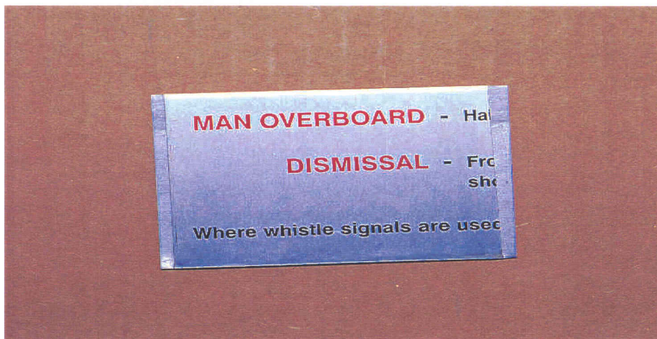
Figure 11: Colored Metalphoto® label plates following environmental exposure. There is no fading or loss of clarity of the printing on these labels.
