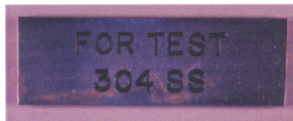
Figure 4: Monel 400™, 316 and 304 stainless steel label plates showing running rust from engraved areas most likely due to iron particle contamination of the surface from engraving tooling.
