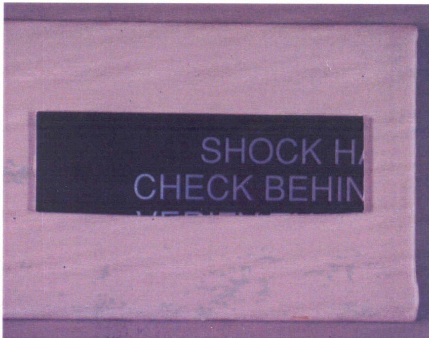
Figure 10: Metalphoto® anodized aluminum label plates with 3M™ Series 1160 Premium Protective Overlay Film before (upper) and after (below) environmental exposure.
